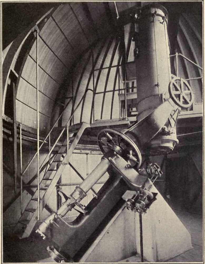
FIG. 139.—Gerrish Drive on 24 inch Reflector.
